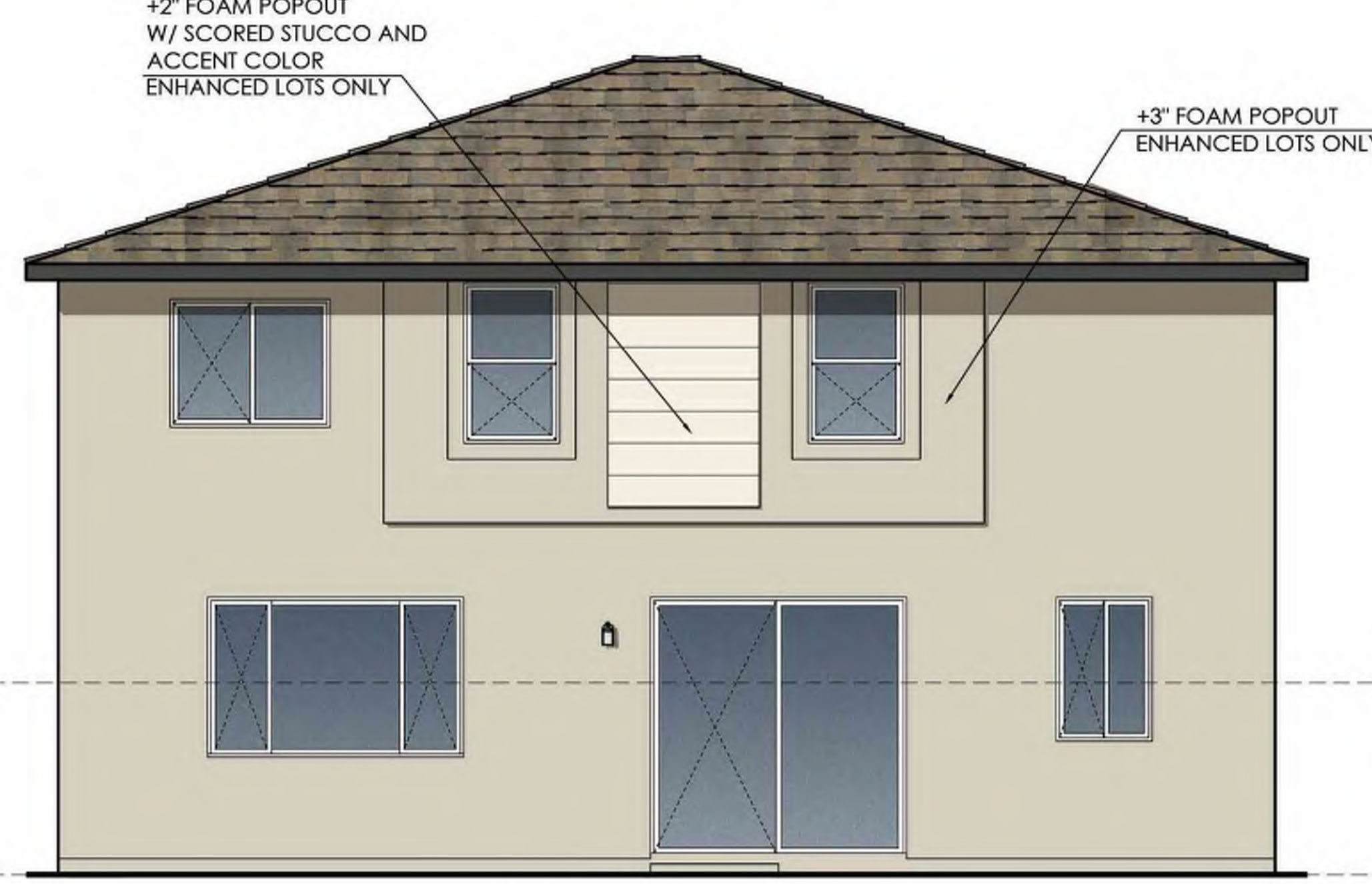
Rear Elevation "Enhanced"
