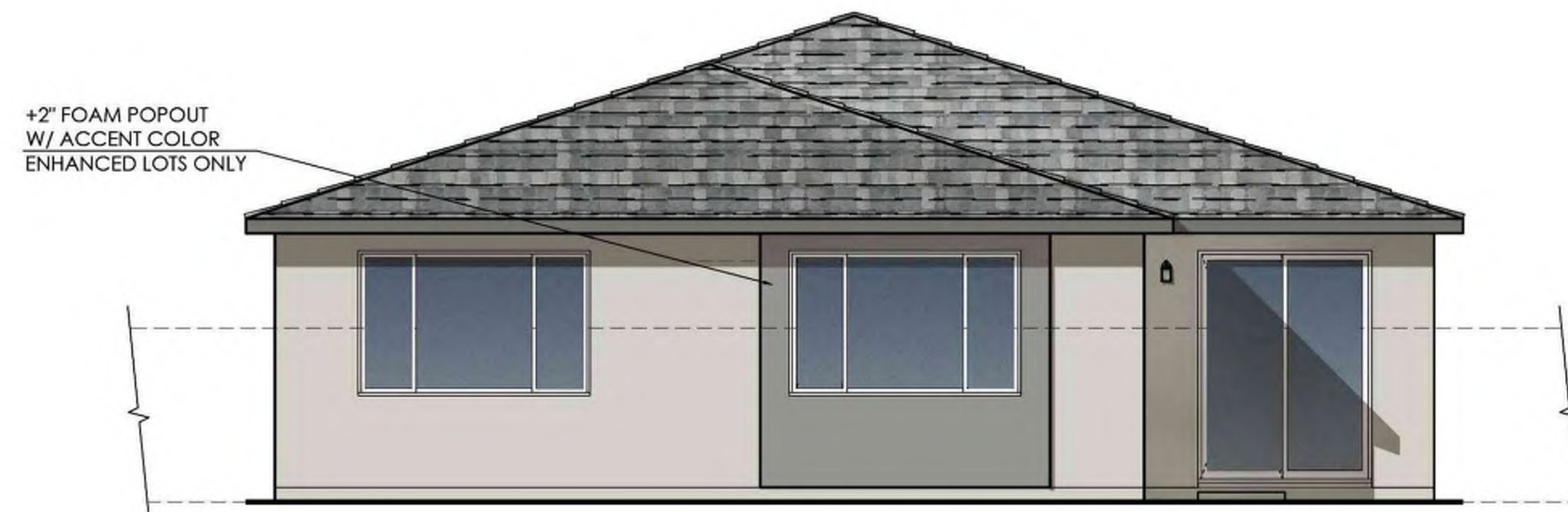
Rear Elevation "Enhanced"
